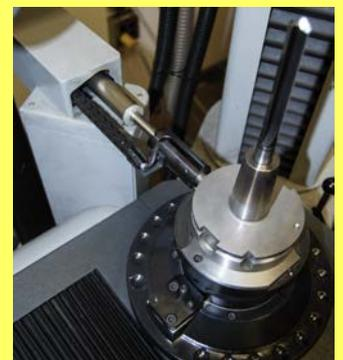
Separate read/write station for manual reading and writing the tool ID chip.
